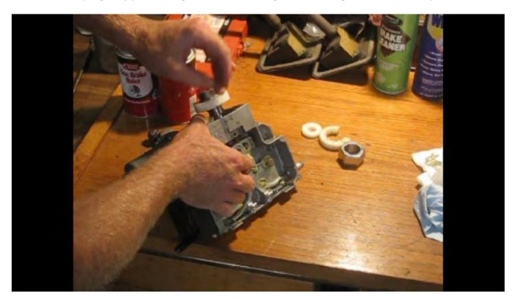
Reinstall the retainer for the shaft with T20 Torx screw.
