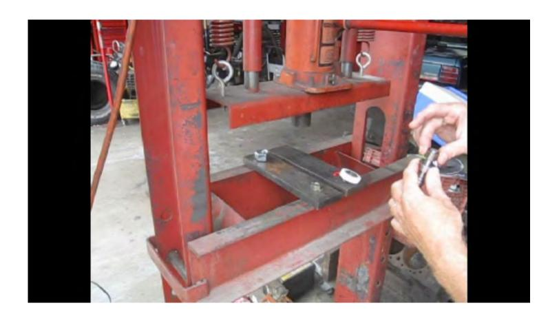
Before installing the new gear apply a small amount of grease to the bushing/bearing section. Press on the upper collar, being careful not to install too tightly as to not bind the movement.
