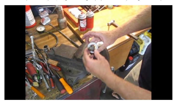
Using a 7/8" socket and a bench vise press the metal gear out of the plastic gear.
