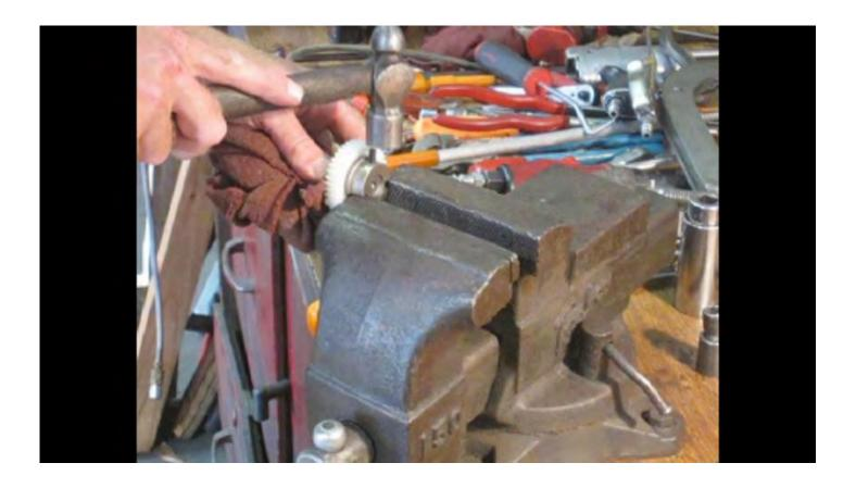
Reinstall the main shaft with the new gear: pull up on the internal mechanism and screw the shaft in until it stops, gently press straight down until the gears mesh together and are fully installed.
