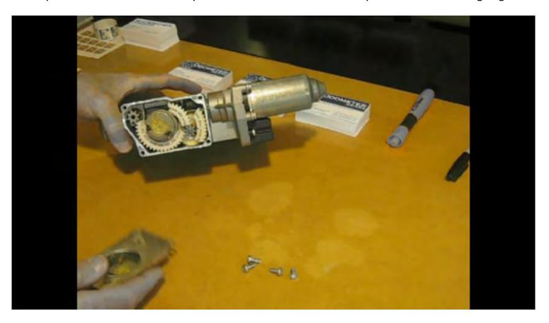
Next remove the T20 Torx screw for the retainer that secures the metal shaft.
