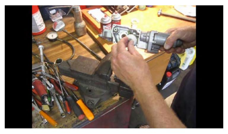
Now press together the parts on the larger shaft in the reverse order removed. Make sure to fully seat each part.
