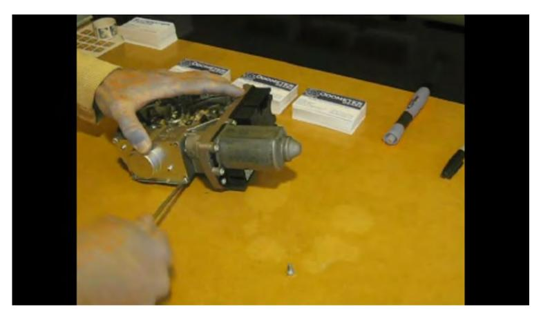
Once you remove the four screws you can remove the cover. Inside you will see the damaged gears.
