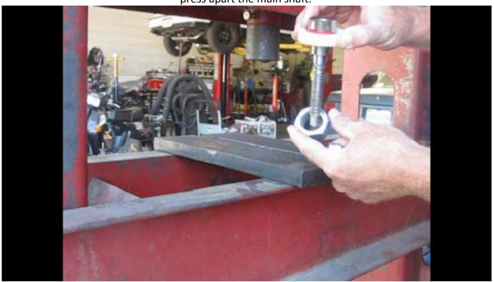
You want to center the narrow press tool or ¼" extension on the center of the shaft.
