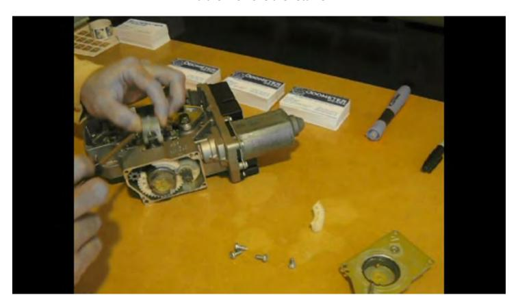
Next unscrew the main shaft that the large gear was on. Also remove the smaller gear, this just pulls straight out.
